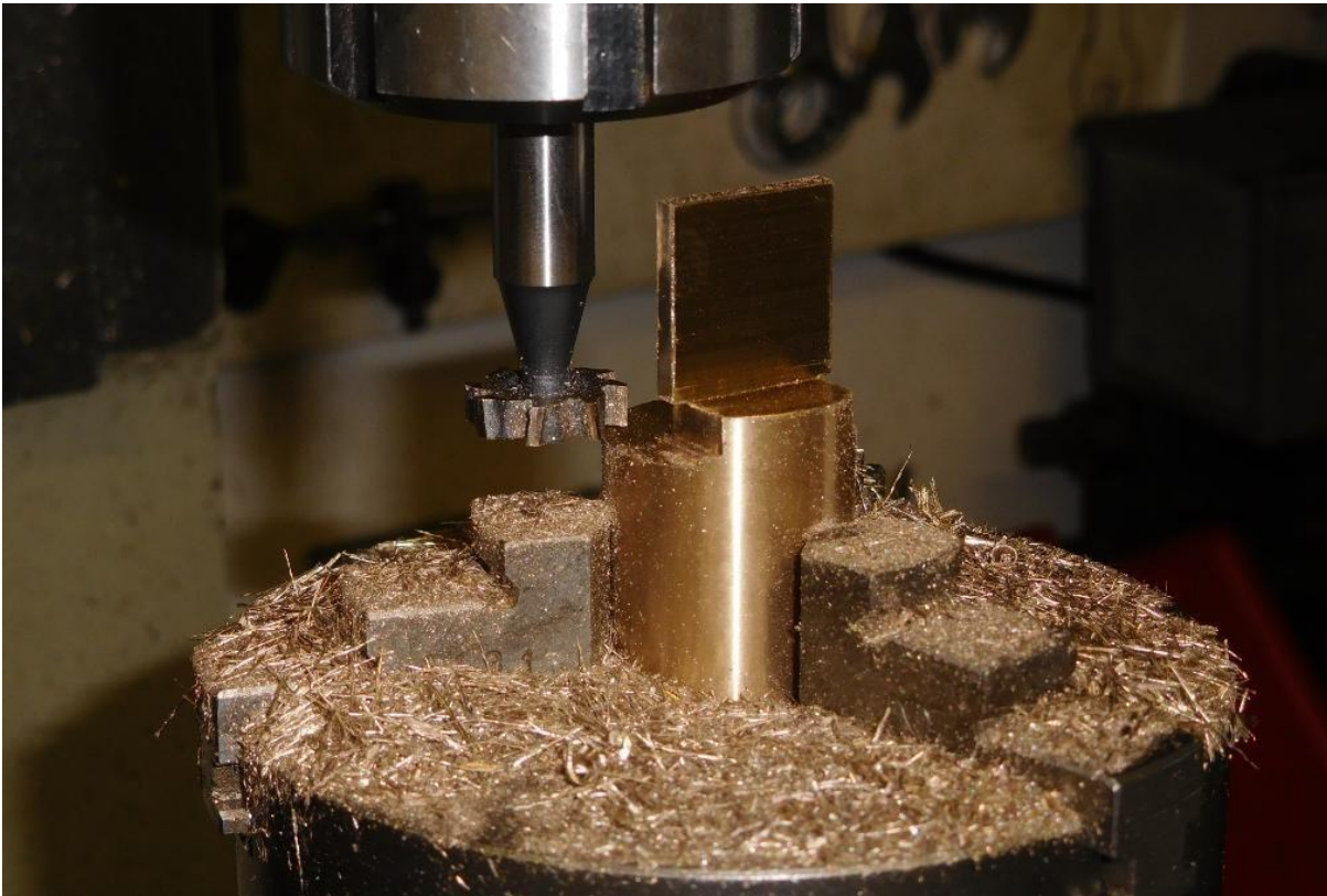
10mm slot drill used to form a mating surface for a piece of 10mm brass to be brazed in later, and holes drilled to suit the cap piece.
