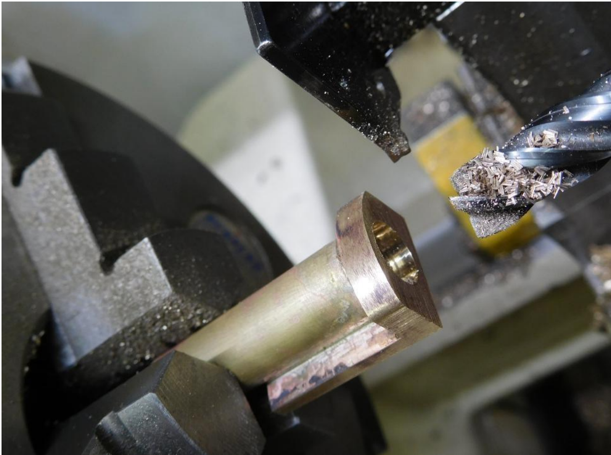
Securing holes drill, cap made; job done.
