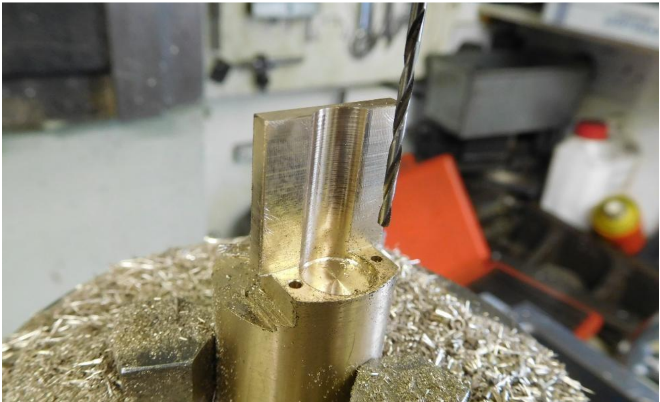
10mm slot drill used to form a mating surface for a piece of 10mm brass to be brazed in later, and holes drilled to suit the cap piece.
