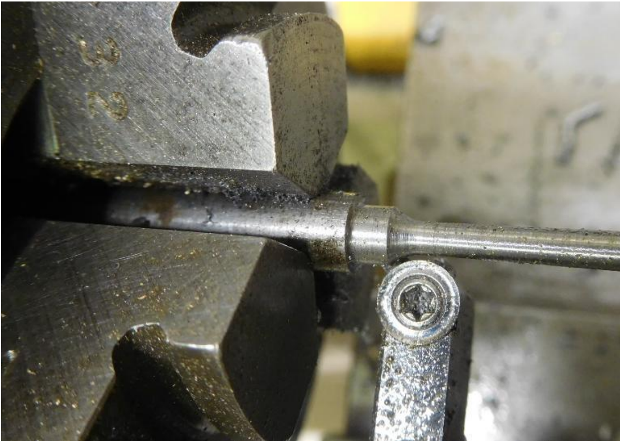
Top pip being formed – this fits in a hole in the cab beading.
