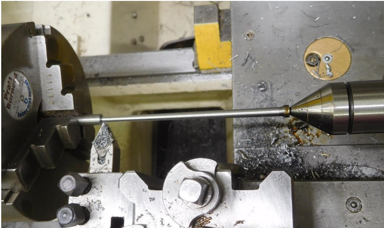
Upper parallel diameter turned to size:
