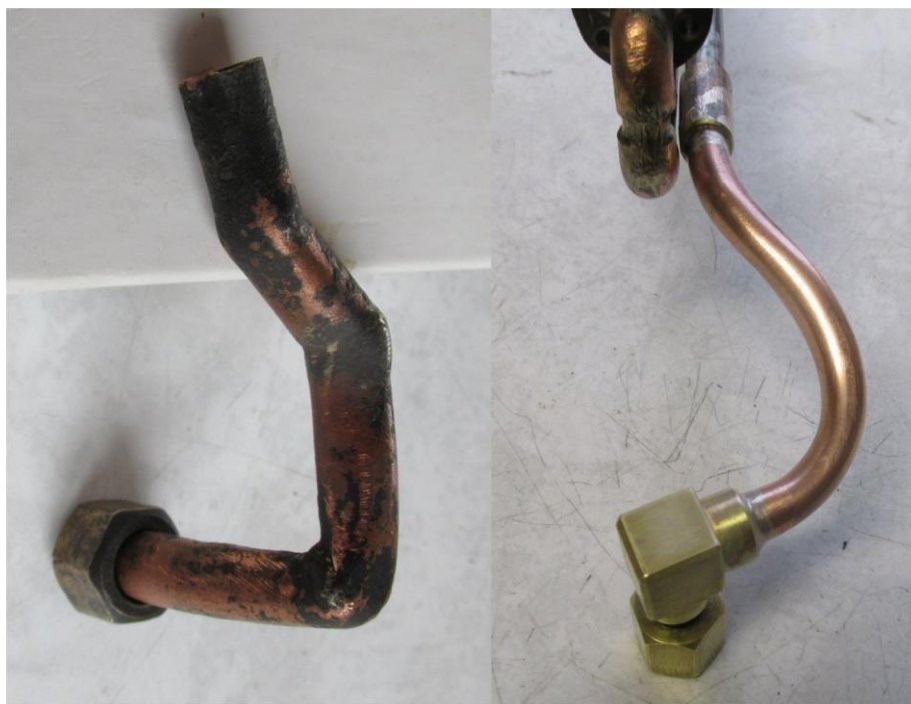
"Before" and "after" super-heater extension pipe
