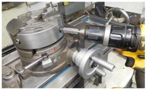
The photo shows the idea; in this case I had no square bar of the correct AF size, but machining a square on an existing square is easier than starting from round bar. In the photo there is limited access to the chuck jaws to use the normal chuck key, so the Power Solution was much better!
