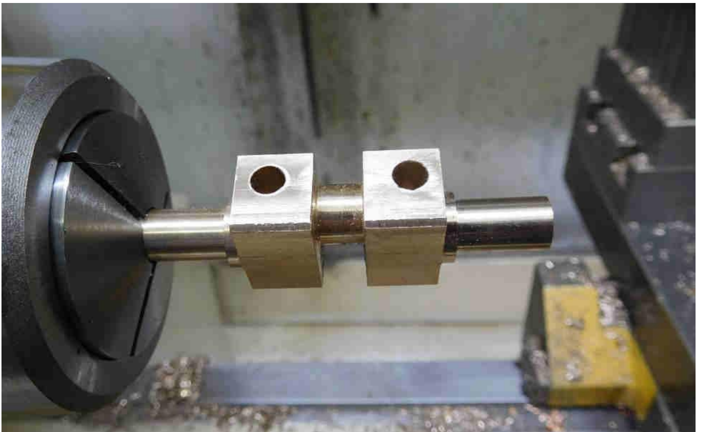
End threaded; note I've made these bosses over-long so I can machine away the centre holes later.
