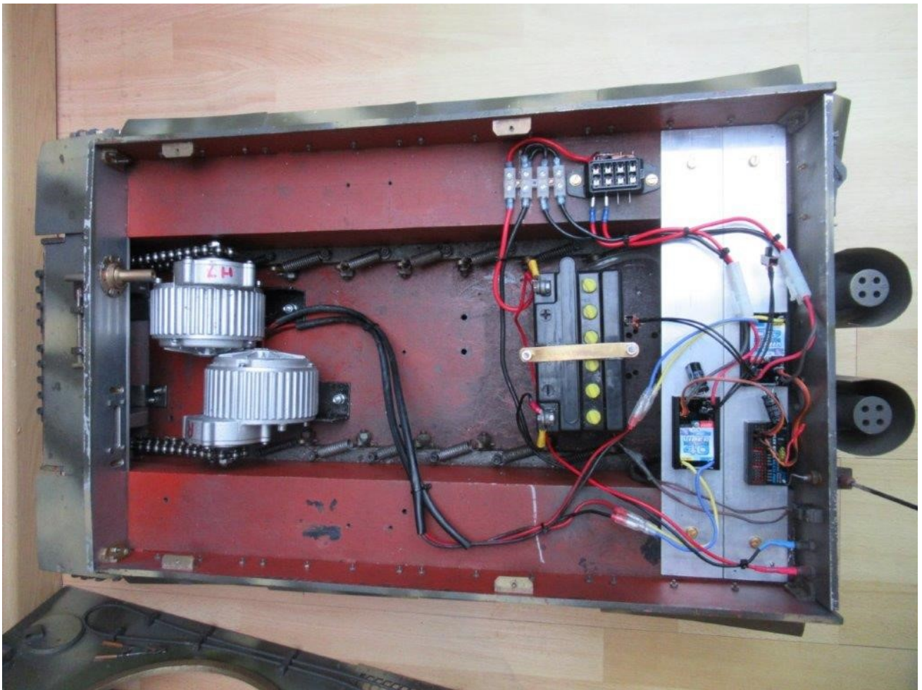
Speed Controller and Fuse Holder Wired Up
